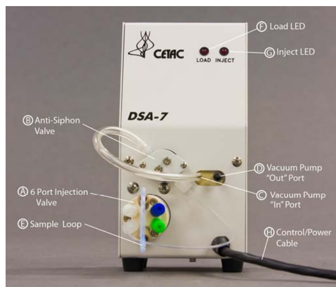
Figure 1. DSA-7 Discrete Sampling Accessory
