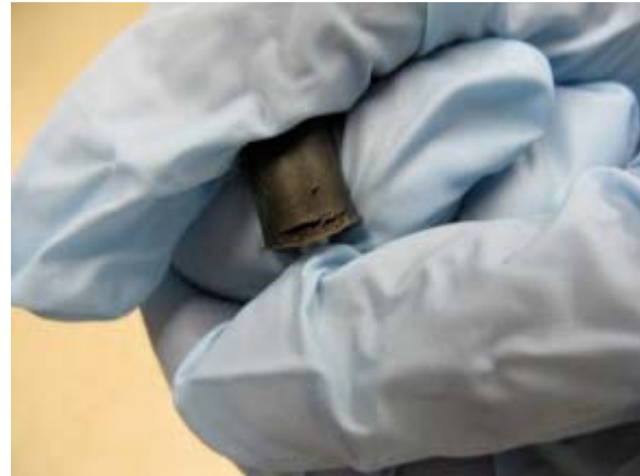
Degrading (cracking) mount
