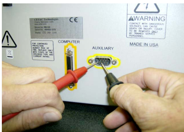
Using a voltmeter on auxiliary pins 6 & 7
