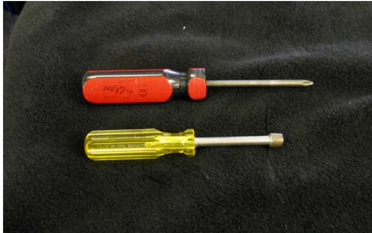
Tools needed: #2 Phillips screwdriver 11/32 Nut driver or socket
