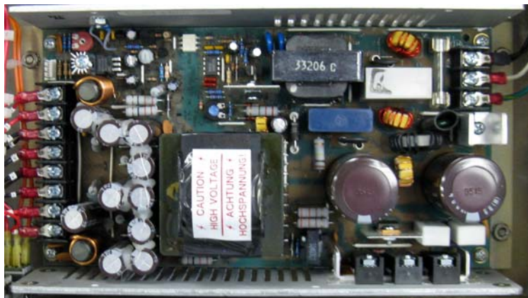
Part to be replaced SP5432 Power Supply U5000AT+
