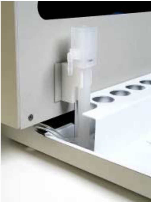
Figure 1-4. View of rinse station.
