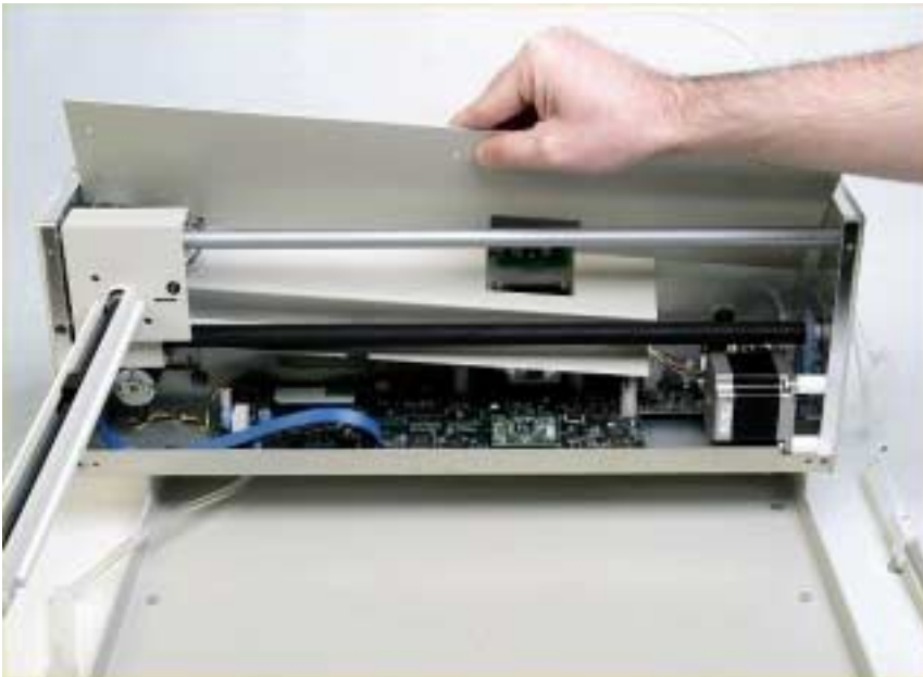
Figure 1-10. Removal of inner shield.
