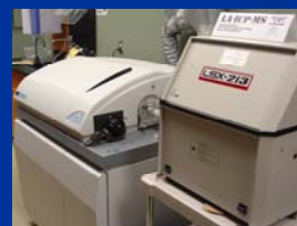
Figure 2. LA-ICP-MS interface consisting of a CETAC Technologies LSX-213 laser ablation system and a PerkinElmer ELAN 9000 ICP-MS instrument.
