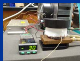
Figure 4. Sub-zero cooling cell (Hyphenated Solutions, Jonesboro, AR) cooled to -30°C. The cell was specifically designed for LA-ICP-MS using CETAC laser ablation systems.
