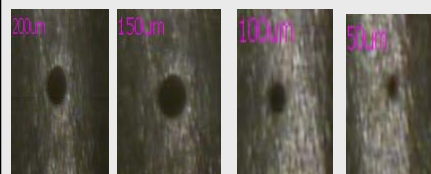
Ablation craters using 266nm laser. Spot sizes 200µm, 150µm, 100µm and 50µm
