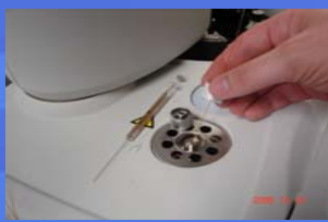
Figure 3. Placement of fused silica transfer capillary through injector nut and septum and into injector liner.
