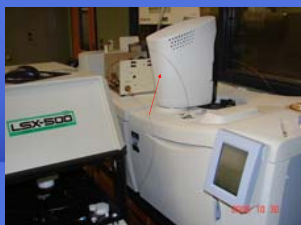
Figure 1. LSX-500, GC-MS, and fused silica transfer line (red arrow).
