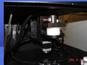
Figure 2. Specialized low volume (5 cm 3 ) sample cell specific for LA-GC studies.
