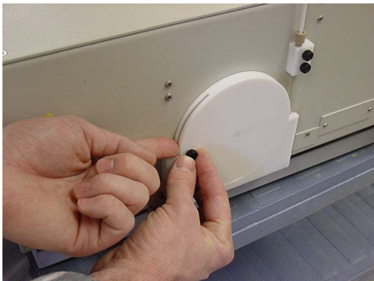
Figure 1-9. Securing cable to rotor (PEEK cable).
