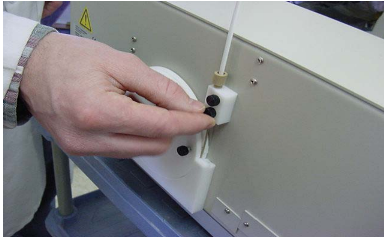
Figure 1-6. Securing block to back of autosampler.
