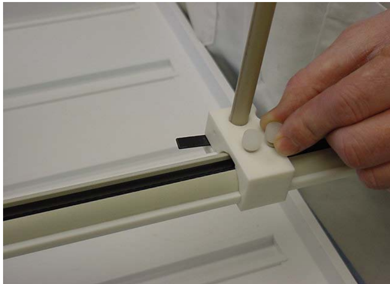
Figure 1-5. Securing z-drive assembly onto autosampler arm.
