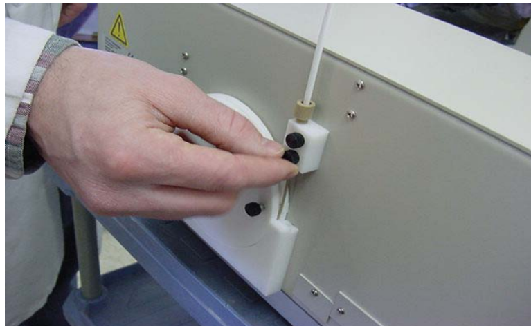
Figure 5 Securing block to back of autosampler.
