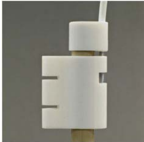
Figure 7 View of gap between probe bracket and cap (carbon fiber style Z-drive assembly).
