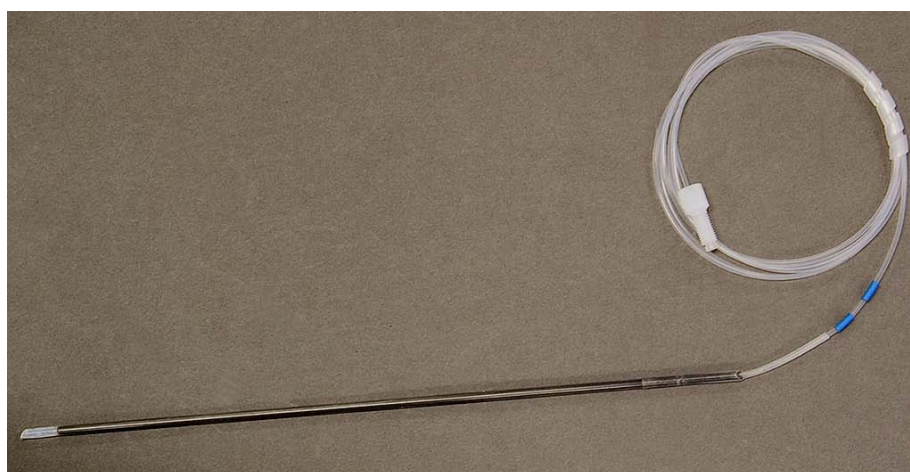
Figure 3-9 Double Blue Bands Identify the 1.0mm I.D. Sample Probe (carbon fiber probe shown is standard equipment)
