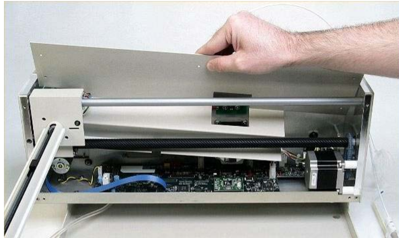
Figure 2-9 Removal of inner shield (ASX-520)
