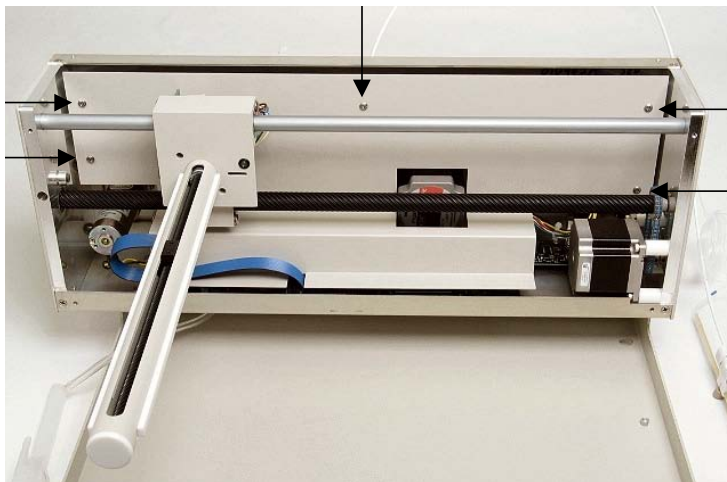
Figure 2-8 View of inner shield inside the ASX-520 autosampler
