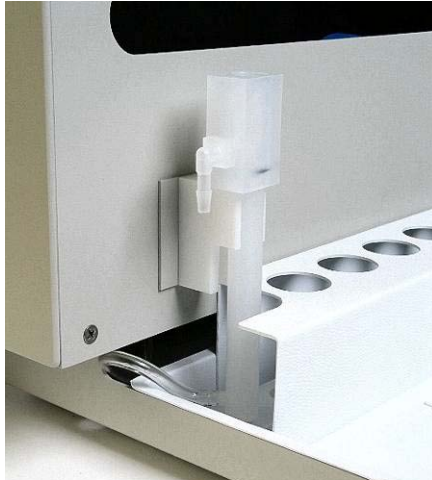
Figure 2-3 View of rinse station
