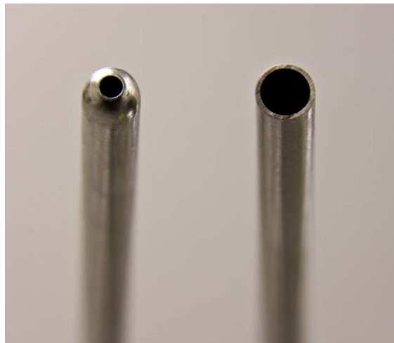
Comparison of new beveled-tip probe (left) to the flat-tip probe.
