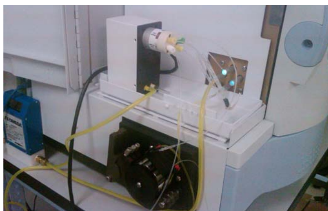
Figure 2. ASXpress™ plus with PerkinElmer Optima series ICP-AES
